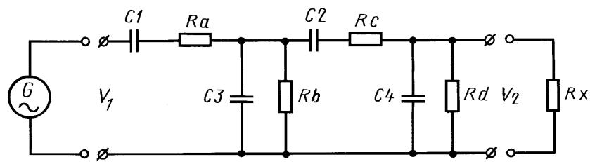
$$(R_a + R_b) \cdot C_1 = (R_c + R_d) \cdot C_2 = 5 \text{ мкС};$$
