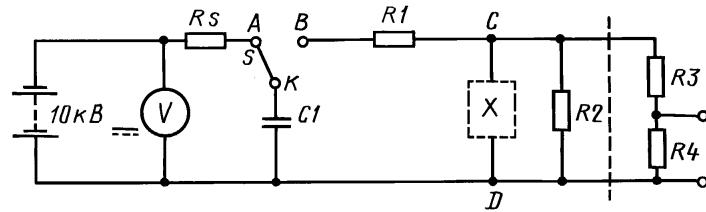
$$C_1 = 1 \text{ нФ}; R_1 = 1 \text{ кОм}; R_2 = 4 \text{ кОм}; R_3 = 100 \text{ МОм}; R_4 = 0,1 \text{ МОм}; \\ R_s = 15 \text{ МОм}$$
