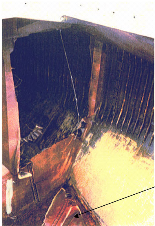
Photograph 1 Collapsed and detached transverse bulkhead
